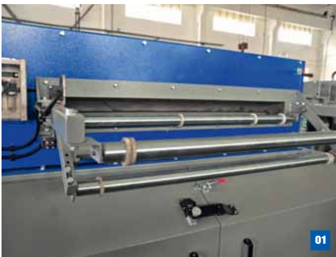
01 GRF granulator with roller feeding system
