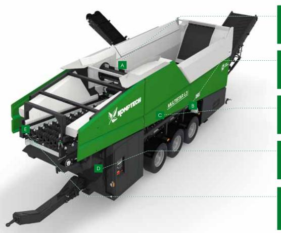
Hopper with scraper conveyor and active metering drum
