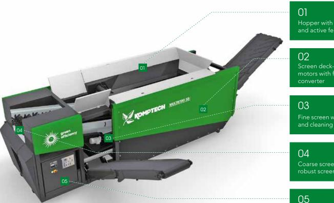
Hopper with scraper conveyor and active feeding drum
